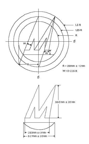
The dimensions are changed to W=0.225R minimum and 0.40R maximum. Height of M= 350mm+/- 25mm and the width of Half Moon M=327 +/- 65mm.
