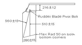
3.7 The dimensions of the **rudder** blade shall conform with the diagram. The **rudder** blade shall be not more than 14mm thick and the thickness shall not vary by more than 1mm to within 25mm of its edges with the exception of hollows or cavities of not more than 2mm in dimension and holes for fixing.
